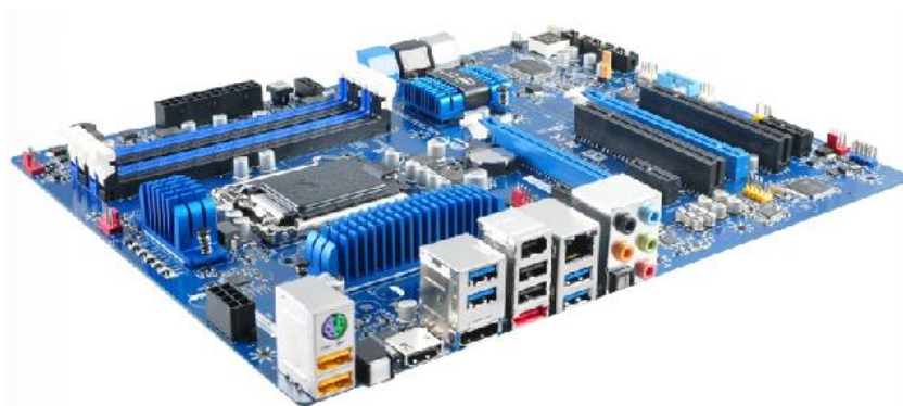
Figure: the Z77 Motherboard – the i-series CPU has made the NorthBridge chip obsolete.
