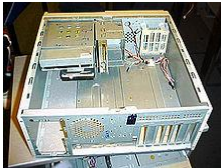
Figure: shows a stripped ATX desktop case. The motherboard will lie flat on the bottom, against the right panel, with peripheral connectors protruding through the rear panel, drive bays at the top and front, and the power supply at the top and rear.
