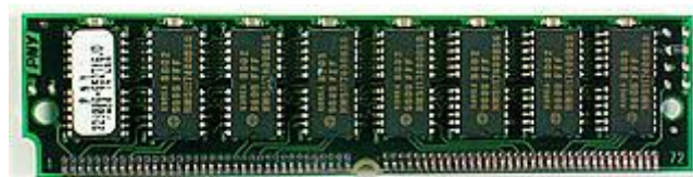
Figure: A RAM Memory Module.
