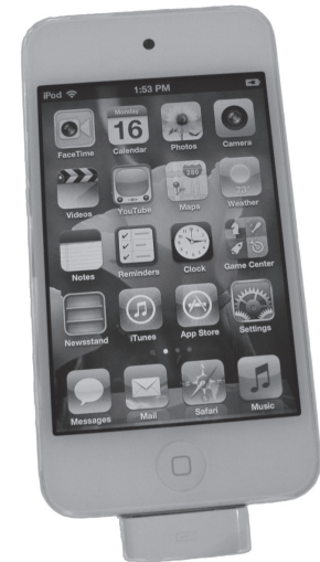
Figure 3.8 The iPod is also a popular storage device. In addition to holding hours of music and video, the iPod can plug into a USB port to record data for transport.
