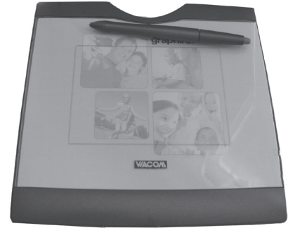
Figure 3.22 Artists and designers use graphics tablets and a stylus pen to input drawings for further editing.
