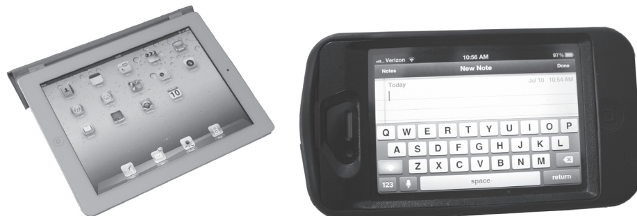
Figure 3.7 With the miniaturization of today's mobile computing devices, the peripherals may not seem so distant. Smartphones and tablet computers embed display and input into the single system device.
