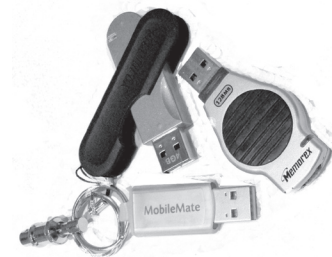
Figure 3.17 Solid-state storage devices have a variety of names. Memory stick, thumb drive, and travel disk are commonly used. The standard name is USB flash drive or “UFD.”
