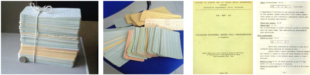
Fig. 1– Left: bundles of cards used for use with computer: old source program and cards with data for elaboration. Dimension reference: coin of one euro. Right: cover and one page of a course on Basic and Fortran languages
