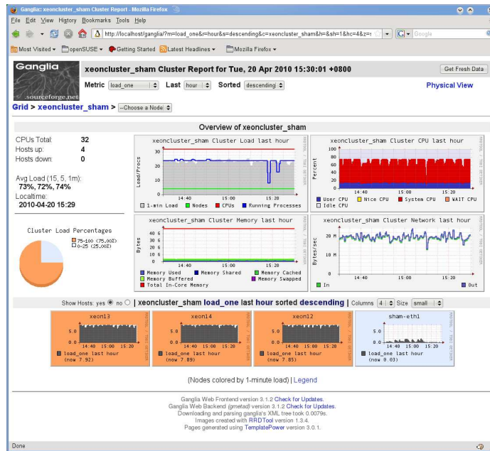
Figure 4.2: The web display of system resource usage monitored by Ganglia.
