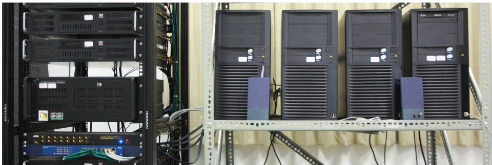
Figure 4.1: The four computers at the right hand side of the picture are the server and the three clients of the high-performance computing cluster. The gigabit switch and the KVM controller are at the lower left corner of the picture. Currently, this Xeon cluster is sharing the gigabit switch and the KVM controller with a Opteron cluster. All other hardware in the picture belongs to the Opteron cluster.
